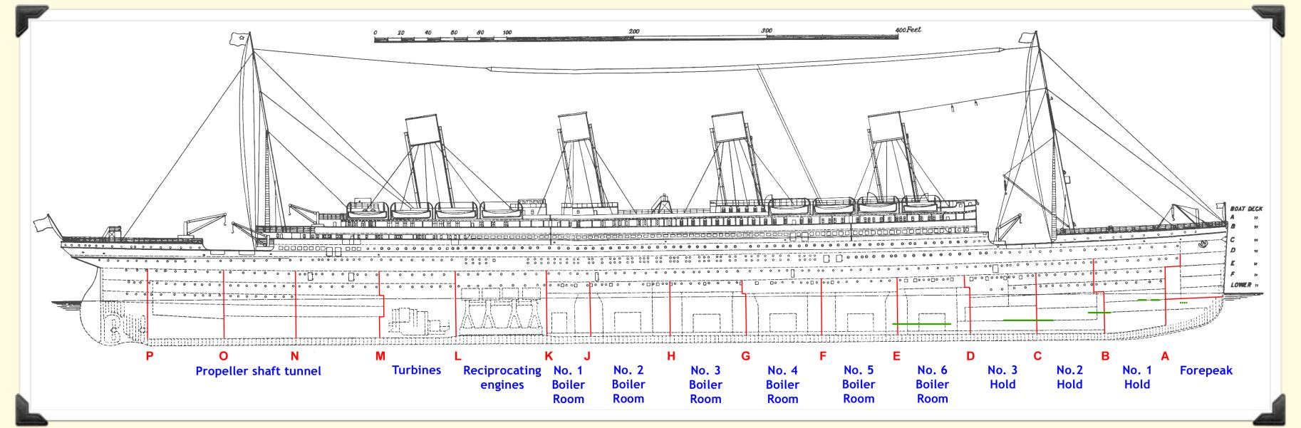
The idea behind the design was that if up to four compartments flooded, the watertight bulkheads (walls) would prevent more compartments from taking on water, keeping the ship afloat to wait for assistance. However the bulkheads were not sealed at the top, allowing one compartment after another to flood as they became full, slowly bringing the bow of the ship underwater. This design flaw was another reason blamed for the sinking of the 'unsinkable' Titanic.
