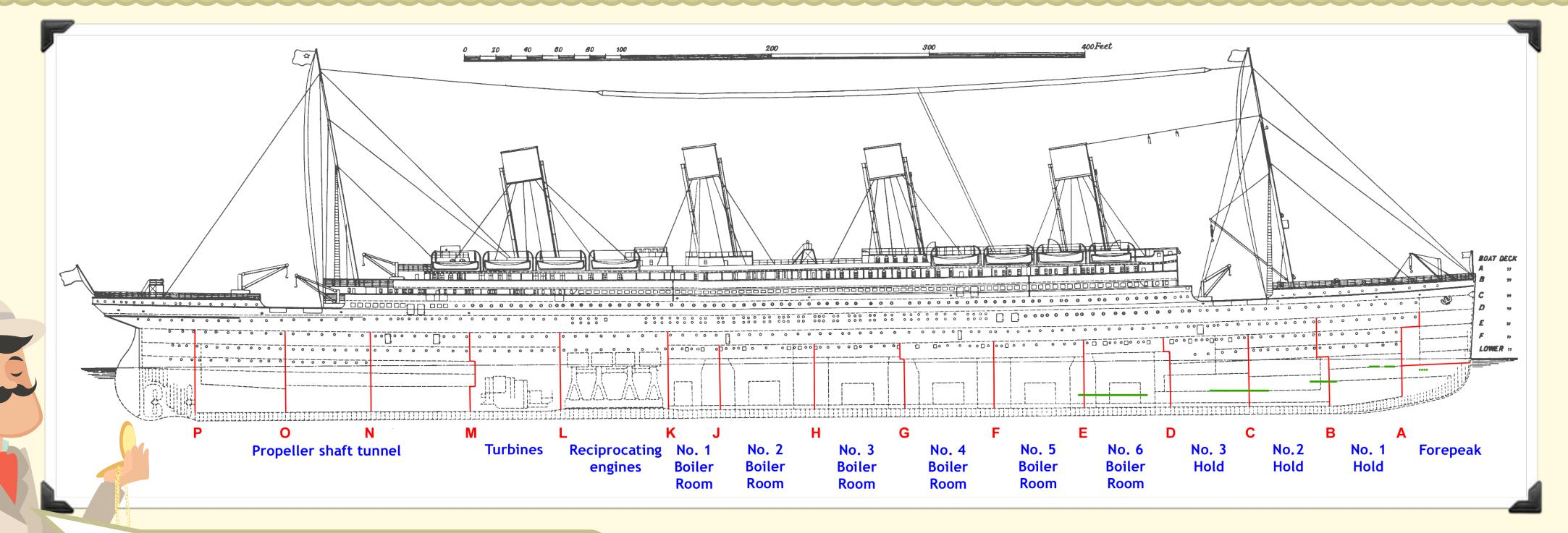
The red lines show the compartment sections. The green lines indicate where the ship's hull split after the collision.
